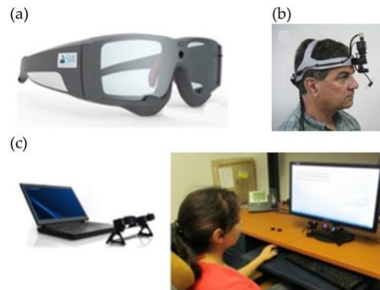
Figure 3.6. Sample of various kinds of eye-tracking tools: (a) eye-tracking glasses [314]; (b) helmet-mounted [315]; (c) remote or table [316].
